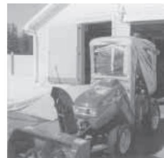
Murray Scea adapted a canvas cab to fit the rollbar cage on his 1998 Honda 1855 tractor. It’s the same color as duct tape so it’s easy to patch.
