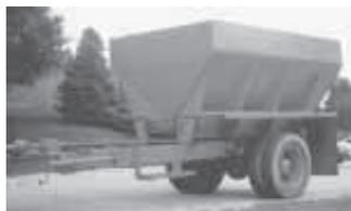
He converted the truck to a trailer by cutting off the cab and adding a hitch and a pto drive. Total cost was about \$1,200.
