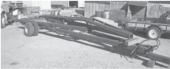
Dual-wheeled, 35-ft. long crane operates off tractor hydraulics and has a 22-ft. long, A-shaped base hinged to back end of rig's frame. Hydraulic cylinders raise and lower base frame.
