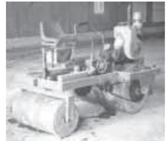
Alvin Wallace's roller is powered by a 2-cyl. Wisconsin engine that drives a combination speed reducer and reverser, which lets the roller run either in forward or reverse. Rear roller holds 100 gal. of water.
