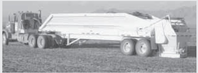
Jace Agee recently built this 10-wheel semi trailer rut filler. It holds 22 yards of material and can travel at highway speeds.
