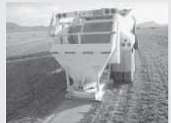
Hydraulic-operated door at back of trailer has a steel compactor plate underneath it.
