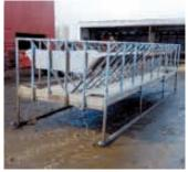
Feeder is 6 ft. wide and 21 ft. long, with a V in the center to hold three 60-in. bales above a wooden bunk.
