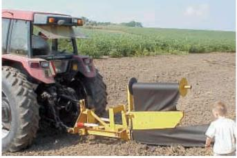
New 3-pt. mounted fabric layer is equipped with a single large shank with a roll of fabric on a horizontal shaft above it.
