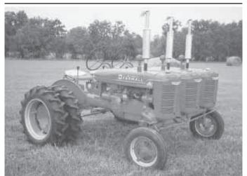
Dewitt Stewart of Bogalusa, La., mounted three Farmall A's together on a frame with a single front axle and a single set of rear dual tires.
