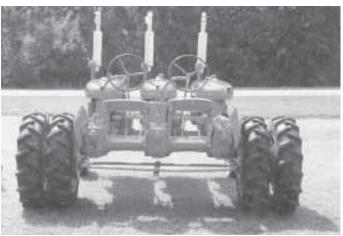
Tractor runs on one, two or three engines in any order. It has two steering wheels and two sets of clutch and brake pedals so Stewart can drive the tractor from either side.
