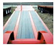
"Rumber" is made of ground-up scrap tires and recycled plastic. Here it was used to make a trailer floor.
