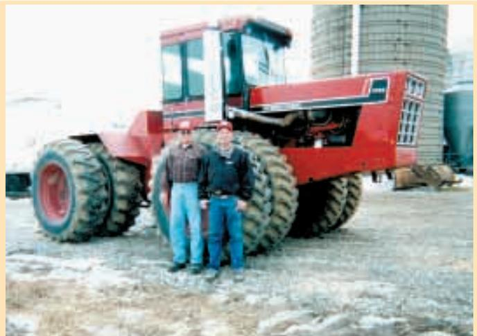
David and Ken Bense replaced the V-8 diesel engine on their 1985 IH 4786 4-WD tractor with a 6-cyl. Cummins 855 diesel engine out of an IH 4070 cab-over semi tractor.
