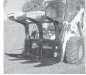
Grapple fork can be used to break up concrete much faster than a jackhammer or other conventional methods.
