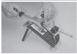
"It removes only a fraction as much metal as a conventional sharpener," says Ben Dale about his new knife sharpener.
