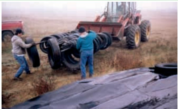
Three 17-ft. lengths of 2 3/8-in. dia. drill stem pipe, spaced about 3 ft. apart, bolt to bucket. Pipes carry about 50 car and truck tires at once.
