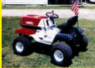
could fix it. I first decided to paint it and, as you can see, I got a little carried away. Then I extended both rear axles and the front spindles. I put big tires all around and made front fenders out of rear fenders from another tractor. I got the 10 hp. motor running and then read an article in FARM SHOW about someone who made a little tractor that ran 45 mph. So I changed pulleys on the transaxle and on the motor so that this little tractor now runs 45 mph and even does wheelies.
