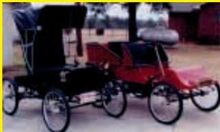
Model "A" Fordmobile. Both have 5 1/2 hp. Honda engines, lawn mower transmissions and differentials. They have heavy 26-in. bike wheels with sprocket and chain drives. The "horseless" carriage has tiller steering. The 1903 model has rack and pinion steering. Both have bodies made of pine and cypress lumber bonded to steel frames. (Ed Beck, Box 8, Hartsville, S.C. 29551 ph 843-332-7398)
