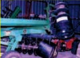
cut two 50-gal. plastic barrels in half and made cutouts along the side for the disk hangers and disk scrapers, then slipped them over the end of each gang. I hold them in place with bungee cords. (Lewis Leon Dick, Mount Hope, Kan.)
