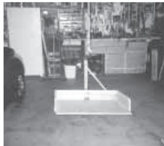
operation by attaching a rod to the winch and using an electric drill to supply the power."
