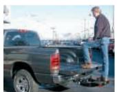
Step provides easy access while still allowing for hitching and towing.
