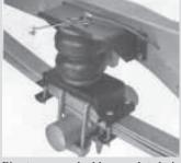
Firestone uses double-convoluted air springs for increased load-leveling and carrying capacities.
