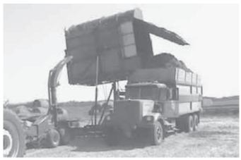
Palechek placed stackwagon box on end, with floor bottom toward tipping side of wa gon. Box is hydrualically raised and tipped on its side to load truck.
