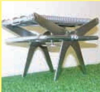
Photo above shows trap in the "set" position. Trap is set by stepping on it until trigger pushes down onto tunnel. Photo at right shows trap after it's been "sprung".
