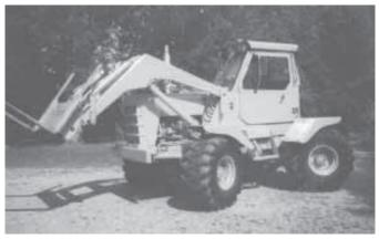
Melvin Putikka used parts from an Army truck's front axles to build this big loader tractor.
