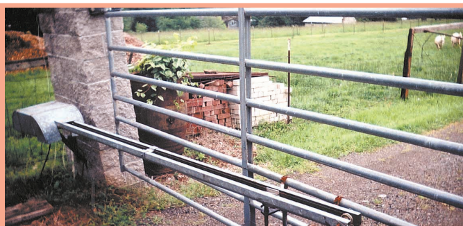
Garage door opener is housed under a 14 by 29-in. cover made from a salvaged heating duct. It's operated by remote control.
