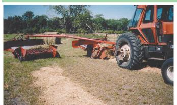
Swath turner consists of two home-built swath turners hooked in tandem on a hydra swing tongue.
