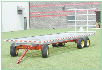
All-steel wagon bed comes with an expanded metal grating floor, stake pockets, and removable back panel. If you want you can mount it on your own running gear.
