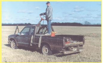
Don Selby made this "trapping truck" by extending the steering wheel and other controls up through the roof.
