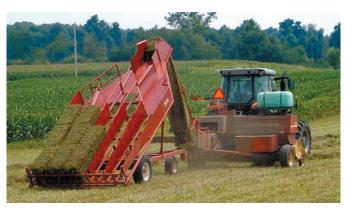
Bale accumulator is built simple with no hydraulics or electronics. It's designed to handle the smaller 32 to 40-in. long bales favored by many smaller hobby farmers.
