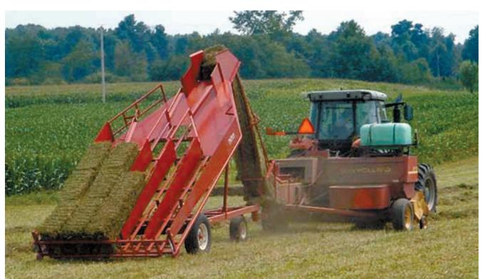
Bale accumulator is built simple with no hydraulics or electronics. It's designed to handle the smaller 32 to 40-in. long bales favored by many smaller hobby farmers.
