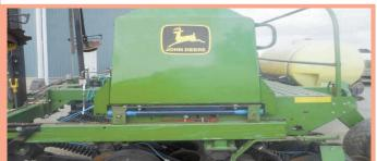
Load bars under seed box are visible from end of drill.
