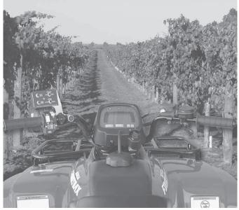
QuadCruise cruise control lets you set a constant speed from 2 to 15 mph. It's especially valuable when spraying or applying fertilizer, says the manufacturer.
