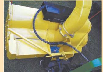
Chute turns 300 degrees, controlled by a small hydraulic cylinder.
