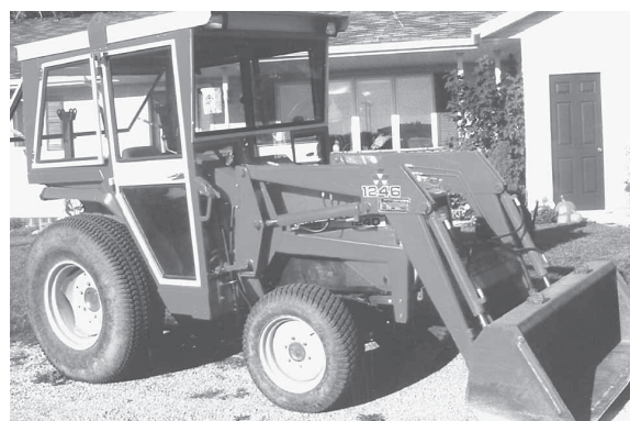
Old 190 AC cab fit Klosterman’s Massey 1240 tractor. He spent about $350 on the conversion.
