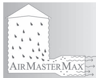
An 18-in. dia. fan mounts in place of existing fan. It pulls down air from the top of bin using a 4 hp electric motor.
