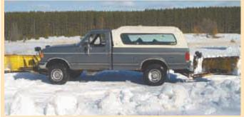
"It lets me plow snow in both directions so I never have to turn the truck around. That reduces my plowing time by half and also saves on fuel," says Alan Strange.
