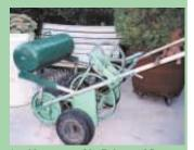
An old rope-start 3 hp Briggs and Stratton engine propels the aerator drum forward. Edwin Ruff says the big gest challenge was gearing down the engine to a slow walk. He used two gear reductions to do that.
