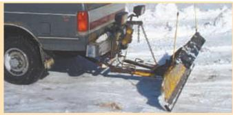
Strange made his own mounting kit for the plow. It's operated by a self-contained battery and hydraulic pump that mount in the pickup bed.
