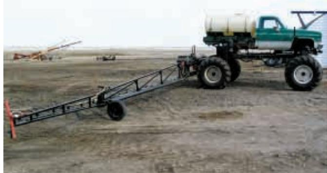
Bernie Denis built this sprayer using a combine drive and a 1981 Chevy 1/2-ton pickup, which he mounted on a home-built frame. It's equipped with an 80-ft. boom.
