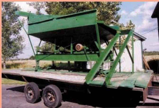
Home-built sand and gravel separator sorts out sand and then bags it. It's equipped with a screen that vibrates at 1,000 times per minute, and has springs on all four legs.
