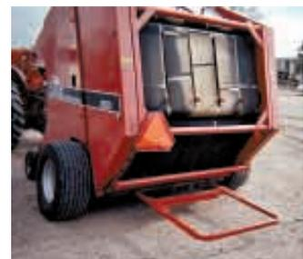
Automatic bale kicker consists of a 3-ft. wide, 4-ft. long metal bracket attached to three big springs. When bale falls onto bracket, bracket lowers to ground. Once bale rolls off, bracket automatically raises up off the ground again.
