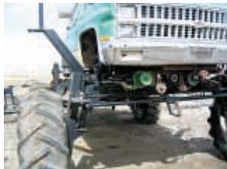
Closeup shows steering mechanism and hydraulic pump.
