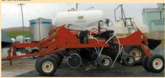
Three-section frame has one rank of coulters, two ranks of standards, a 130-bu. dual compartment seed fertilizer tank, and liquid fertilizer tanks.
