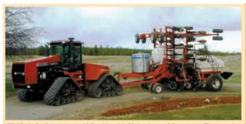
KMCAir Seeder measures 32 ft. wide, with 32 shanks on 12-in. centers. Three-section frame is short-coupled, making it easier to hold on hillsides.
