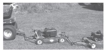
Kornkven's double rake hitch cuts an 80-in. swath and mows lawn twice as fast, while using a lot less fuel.
