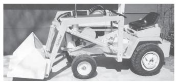
Belt-driven hydraulic pump and reservoir under hood provides lifting power. Three 1 by 2-in. hydraulic cylinders control loader - two to raise and lower the arms and one to tilt the bucket.
