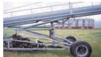
Conveyor is driven by a 400 Ford engine that's coupled to a hydrostatic pump.
