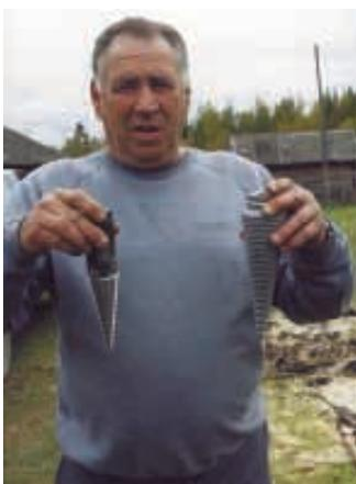
Threaded, cone-shaped wedge fits any 3/4 or 1-in. sq. drive and is held on by a pin that slides through hole in splitter base.
