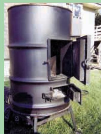
Schreiner used sheet metal and angle iron to build an insulated door and painted the stove black.
