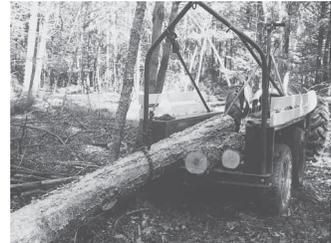
**James Goetsch built this tandem axle walking beam, self-loading log trailer. It's built somewhat similar to big commercial self-loading log trailers used by professional loggers, but on a smaller scale.**
