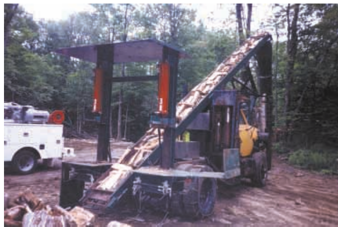
“It splits wood twice as fast as a conventional splitter,” says John Steciak about his self-propelled log splitter. It has two splitting wedges and two work stations on either side.
