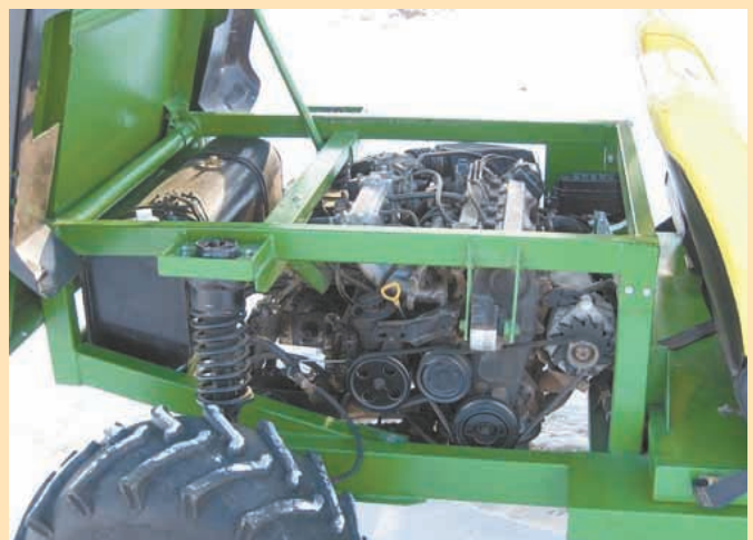
The “IntimiGator”, as Thuerauf calls it, has a homemade dump box that’s designed to be manually tilted back, providing easy access to the rig’s Toyota Corolla car engine.
