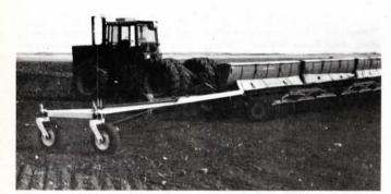
The marker's 14 in. dia. rims keep the horizontal connecting arm level with the ground. Hinged connecting point allows the marker to float to follow uneven terrain.
