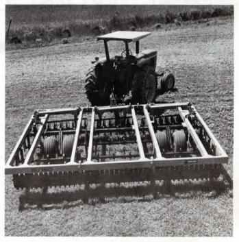
The 15 ft. wide Disc-A-Mulcher is designed to be pulled 8 to 9 mph. Takes a 150 hp or larger tractor. Exclusive rubber cushions on disc section are a key to the new tillage tool's high speed capability.
