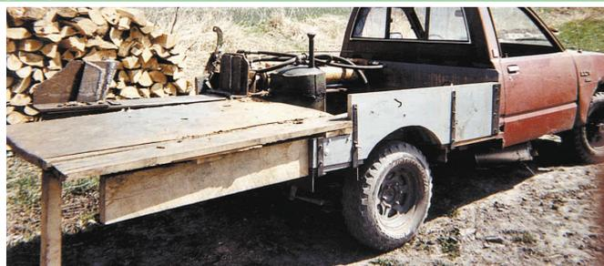
Walter Fifelski uses an old rusted out Chevy 4-WD pickup to power this log splitter.
