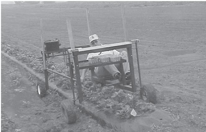
At first Tim Brown tried using a three-wheel pedal cart to pick strawberries, but found it difficult to steer. So he made an electric-powered four-wheel cart that he can steer by simply flipping a toggle switch to go forward or back.
