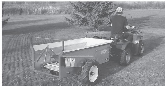
"Unlike other small manure spreaders on the market, you don't have to get off the machine to engage this spreader. The lever is right behind the seat," says Tom Roth, owner of Roth Manufacturing.
