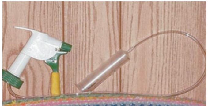
Hand-powered milker is made from a spray bottle, clear plastic tubing, and a syringe.
