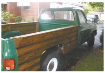
After he couldn't find replacement side panels, Wolters built his own wooden sides for the bed on his Chevrolet 3/4-ton pickup, using pressure treated 2 by 6 pine boards.
