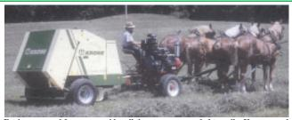
Engine-powered forecart provides all the pto power needed to pull a Krone round
