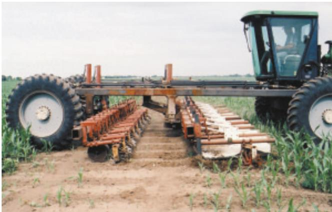
Precision Trac “tool carrier” puts the implement between the front and rear axles for more precise control.
