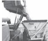
Side dump wagon has a capacity of four tons. It takes less than one minute to dump the wagon and bring it back down.
