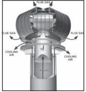
Vacu-Stack's design creates a positive draft that pulls flue gasses up and out of any size chimney. Drawing is of double-walled version.
