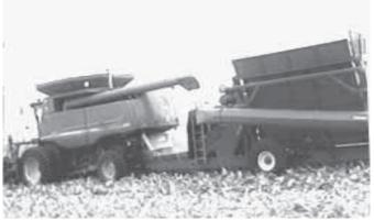
Vernon Flamme's cob collector uses a conveyor to deliver cobs into trailing side dump wagon. System is powered by a diesel engine that direct-drives a hydraulic pump.
