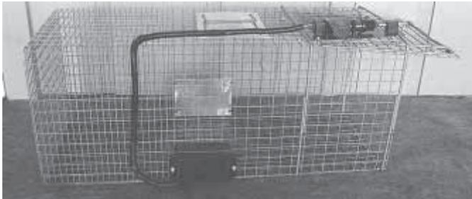
Conversion kit lets you add a laser trigger to an existing live trap. An infrared micro-processor activates a solenoid to release trap door.
