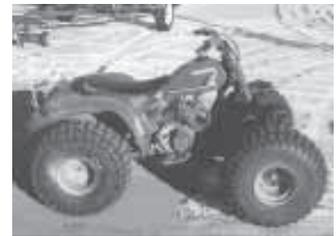
Dwight Keller converted a 1983 Honda 200 Big Red 3-wheeler to four wheels using the front end off an old Toyota car.
