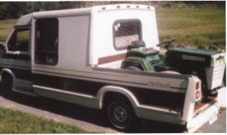
Norman Foellmi converted a 1985 Winnebago Centauri van into a "sleeper pickup" with a 6-ft, cargo box on back.
