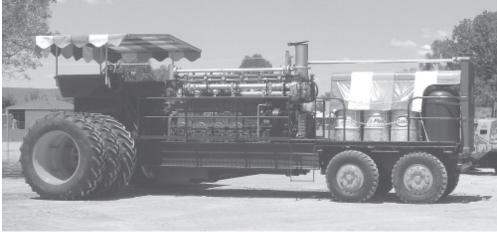
'Ol Rusty is more than 20 ft. wide and 30 ft. long and was built around a Ruston Hornsby 1,000 hp, turbocharged diesel engine (above). Loading and transporting 'Ol Rusty is an art in itself. The canopy and outer wheels are usually removed for highway transport.
