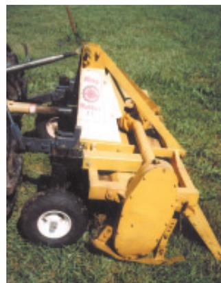
By mounting a 13-in. wheelbarrow wheel on each side of his King Kutter 3-pt. mounted rototiller, Ray Bjorgaard can set the top link on the 3-pt. hitch at the depth he wants and let the tiller float.
