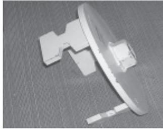
**Beater Claw fits over combine's beater pulley. A 1 7/8-in. nut welded on the Claw lets you turn it with a socket or wrench.**
