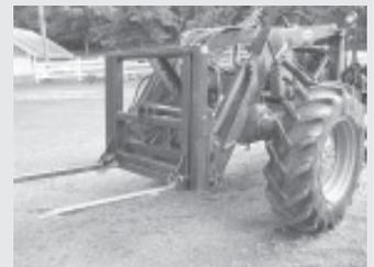
**Special bale fork provides an extra 2 ft. of clearance. A pressure gauge on the lift cylinder shows bale weight within 25 lbs.**
