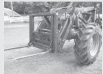
**Special bale fork provides an extra 2 ft. of clearance. A pressure gauge on the lift cylinder shows bale weight within 25 lbs.**
