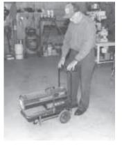
Frank Miller, Beecher City, Ill.: Frank came up with a simple cart equipped with a high rise handlebar, which makes it much easier to maneuver his salamander shop heater. He welded a square box steel frame to the base of the heater. Then he added two utility wheels on back and a small caster wheel on front. The handlebar is made of lightweight pipe.
