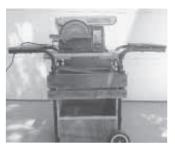
table power sanding machine. First I removed the grill from the stand and replaced it with some wooden boards. Then I mounted a beltdisc sander onto it (any other light shop tools could also be used). I also closed the ends and the back side of the frame with plywood to give the frame more strength, then built a shelf into it to store extra discs or belts. Now I can easily move my sanding machine wherever I need it. It works great.
