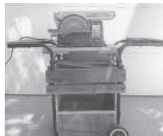
table power sanding machine. First I removed the grill from the stand and replaced it with some wooden boards. Then I mounted a belt-disc sander onto it (any other light shop tools could also be used). I also closed the ends and the back side of the frame with plywood to give the frame more strength, then built a shelf into it to store extra discs or belts. Now I can easily move my sanding machine wherever I need it. It works great."
