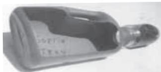
"To make a sorting tray for small bolts, nuts and screws, I cut out one side of a plastic
