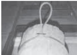
"A V-belt and a large metal washer work good for handling small logs. The loop provides a handle to lift the log."
