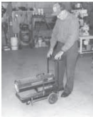
**Frank Miller, Beecher City, Ill.:** Frank came up with a simple cart equipped with a high rise handlebar, which makes it much easier to maneuver his salamander shop heater. He welded a square box steel frame to the base of the heater. Then he added two utility wheels on back and a small caster wheel on front. The handlebar is made of lightweight pipe.
