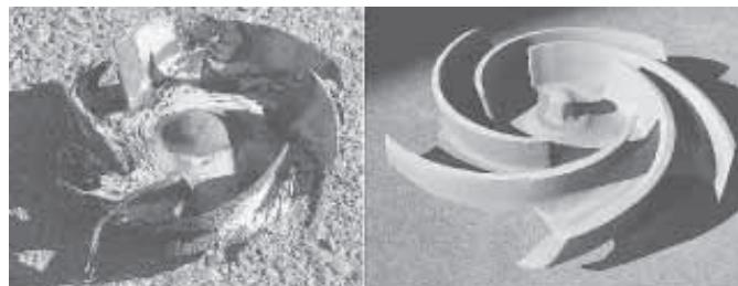
Uncoated impeller, left, lasted 30 days. Impeller at right has been in service 30 days and counting.
