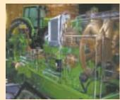
stripped-down tractor at Deere's Agritechnica display made the new tractor easy to understand by having all the new electric-generating components painted in gold.
